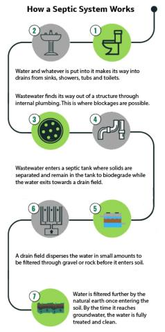
set of drainage pipes layered with crushed stone and topsoil. The layers allow for further filtration of the effluent before it enters the groundwater.
